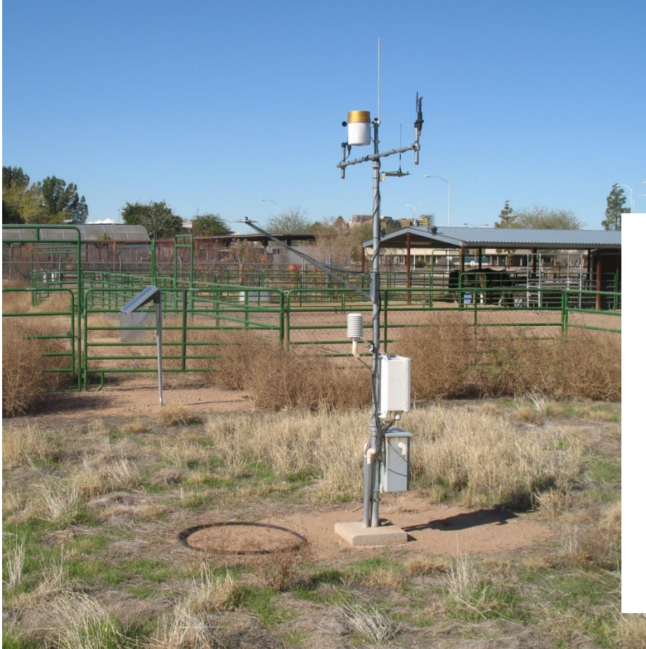
Figure 3. Schematic depicting how ET_0 is determined. Wind, solar radiation, temperature and humidity data from a weather station are used as inputs to the Penman Equation which, in turn, provides the ET_0 value.
